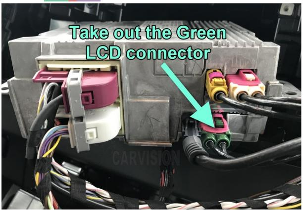
Connect the interface LVDS cables in between like shown below:
